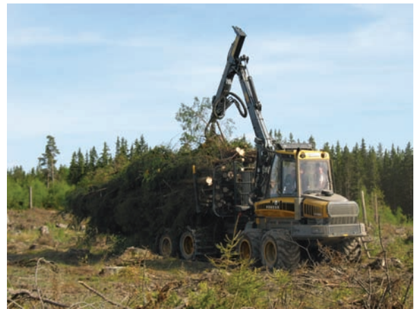
During conventional stem-wood harvest large amounts of energy bound into logging residues are left at site. Today more and more of this resource is utilized. The picture showing a forwarder transporting logging residues. Photo: Ola Lindroos
