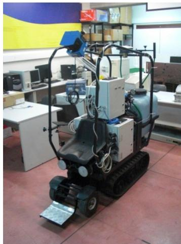
*Figure 7: The U-go robot with the prototype of the automatic electrical sprayer*
