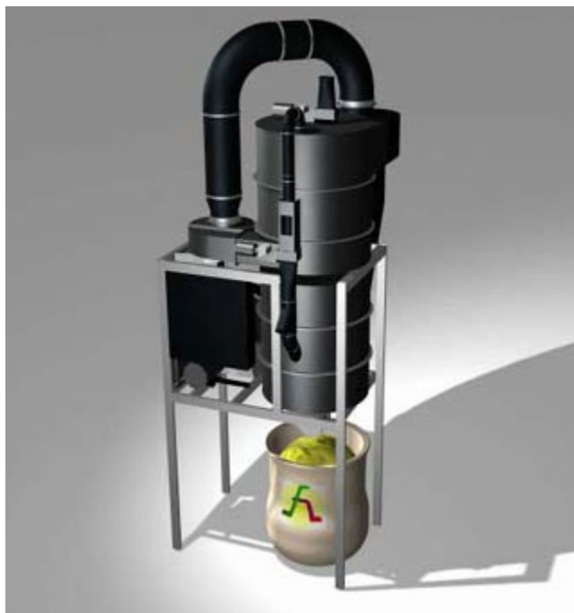
Fig. 4. A CAD drawing of the tested large-scale continuous treatment system operating at 1.3-2 tons/h capacity. The seed flows through the rectangular heating channel bent to a spiral-formed circular treatment chamber at the upper half of the device and then down through the similarly circular cooling chamber before it is filled into a 700 kg bag. The height of the system is about 4 m. (Published with the kind permission of Acanova AB, Sweden).
