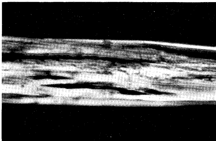
Fig. 22. Cavity-like degradation pattern in a viscose fibre (90 % stretch). Polarized light; Magn.: 830: 1.
