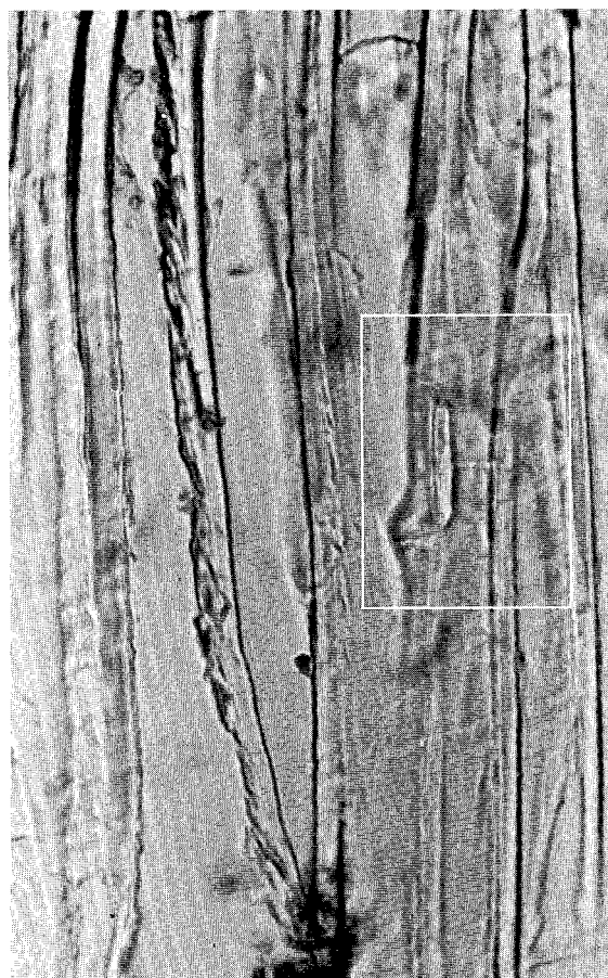
Figure 6 Cavity formed in birch wood fibre by Allescheria terrestris with three bore-holes, one in each end of the cavity and one in the centre of the long edge. Approx. 875 \times .
