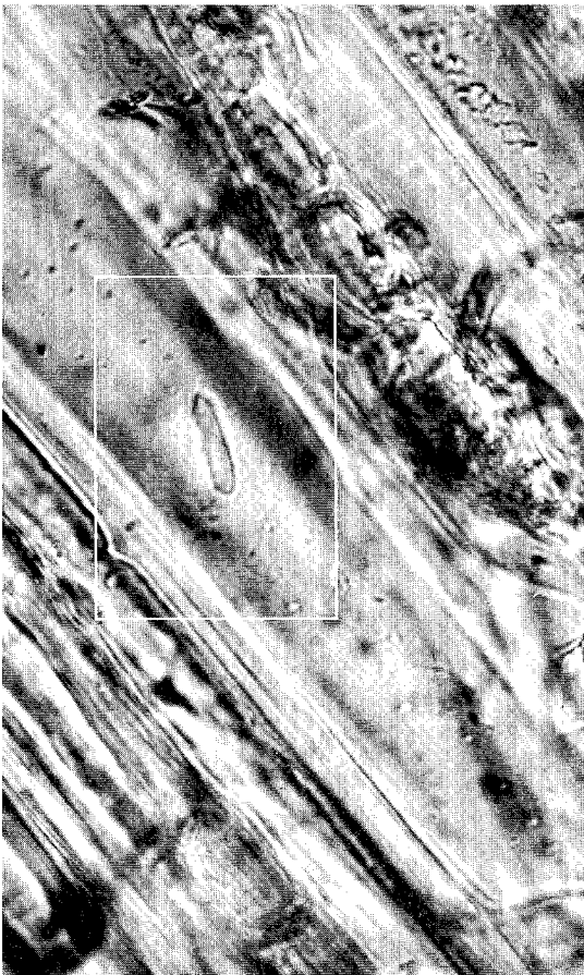
Figure 8 A cavity formed in a birch wood vessel after 100 hours of attack by Allescheria terrestris . Approx. 875 \times .
