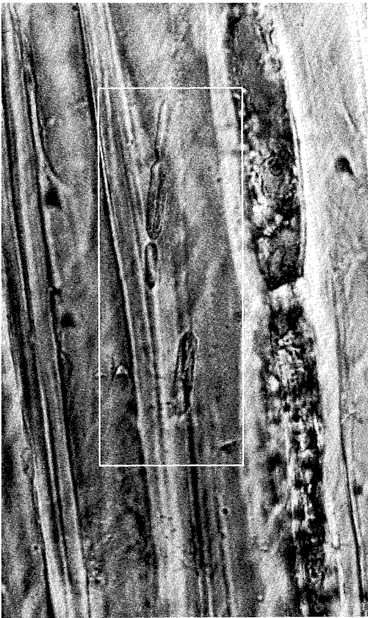
Figure 11 A. Cavity chain with three cavities formed by Allescheria terrestris after 70 hours' attack of birch sapwood impregnated with a 0.6 per cent solution of ammonium tartrate.
