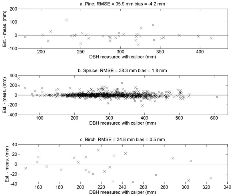
Figure 5. The residuals of DBH estimated from TLS data versus manually measured DBH for pine (a), spruce (b), and birch (c).
