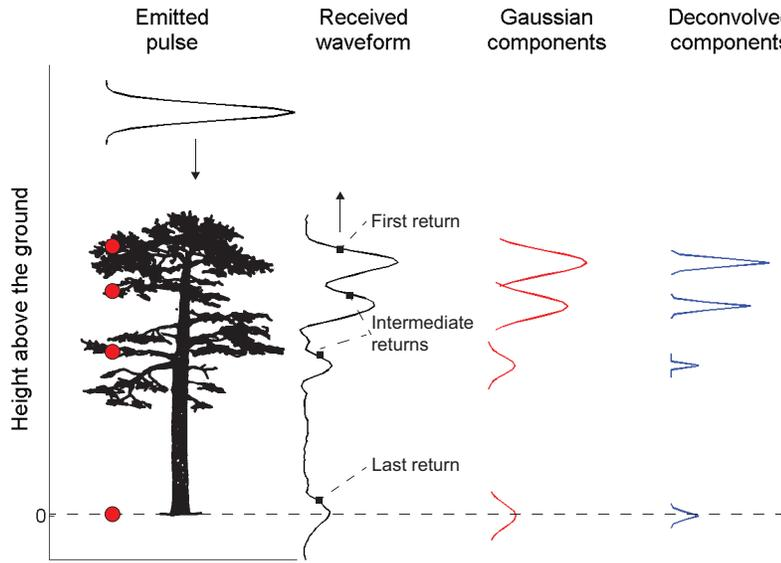
Figure 1. The emitted pulse is reflected from different surfaces, resulting in a waveform that can be used to derive discrete returns. The waveform may also be decomposed into Gaussian components and deconvolved to obtain more detailed information about the reflecting surfaces.
