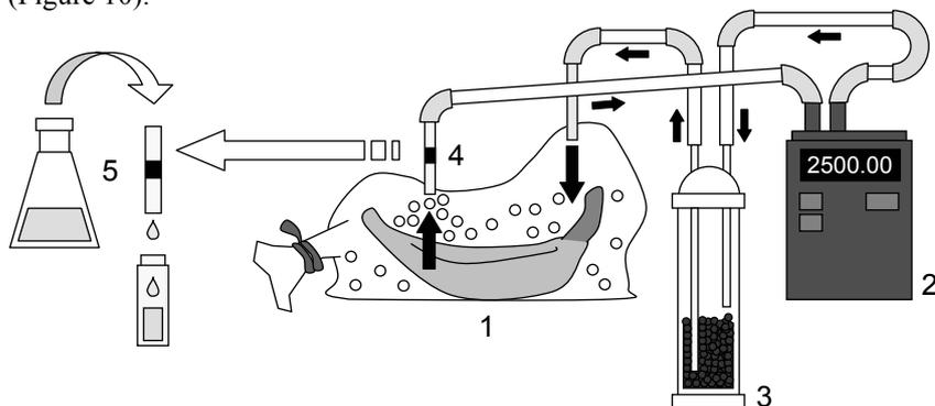
**Figure 10.** Head-space collection of odor volatiles. The volatile source (1) (in this case a banana) is encapsulated in a plastic bag; air is pumped (2) into the sampling bag after purification (by passage through active charcoal) (3). The pump then evacuates the air inside the bag through a charcoal filter (4), which traps the odor volatiles. The collected volatiles are then flushed from the filter with a solvent (hexane or methylene chloride) (5).
