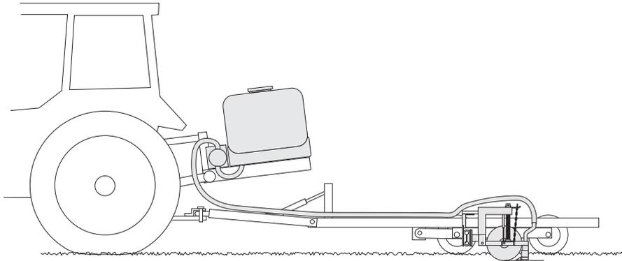
Fig. 11. Trailer with a slurry tanker used in field experiments.
