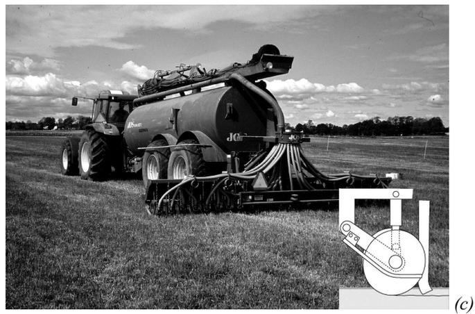
Fig. 3 a-c. Application methods used; (a) pressurised injection (PI); (b) shallow injection 1 with open slots; V-shaped disc tine (SIO1); (c) shallow injection 2 with open slots; tine consisting of two angled disc coulters (SIO2).
