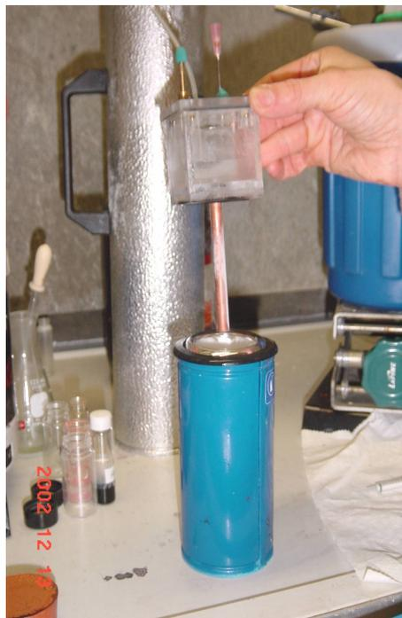
*Fig. 11.* Equipment used for measurement of X-ray absorption in the EXAFS experiments. (Photo: Magnus Sandström)
