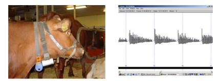
**Figure 3.** Noseband sensor, head collar and recorder as fitted to a cow (left), and the jaw movement amplitudes during rumination as displayed in GRAZE<sup>®</sup> 0.8 (right).
