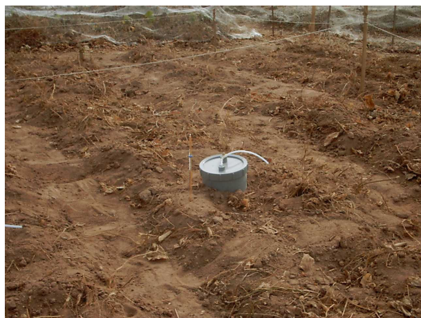
Figure 10. Picture of vented closed chamber system. Next to the chamber a thermometer is inserted into the soil. Photo: K. Röing.
