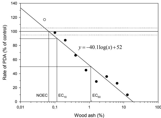
Figure 15. Changes in soil PDA after application of different rates of wood ash. Filled symbols represent data included in the linear regression.
