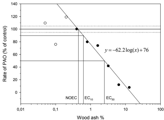
Figure 14. Changes in soil PAO after application of different rates of wood ash. Filled symbols represent data included in the linear regression.
