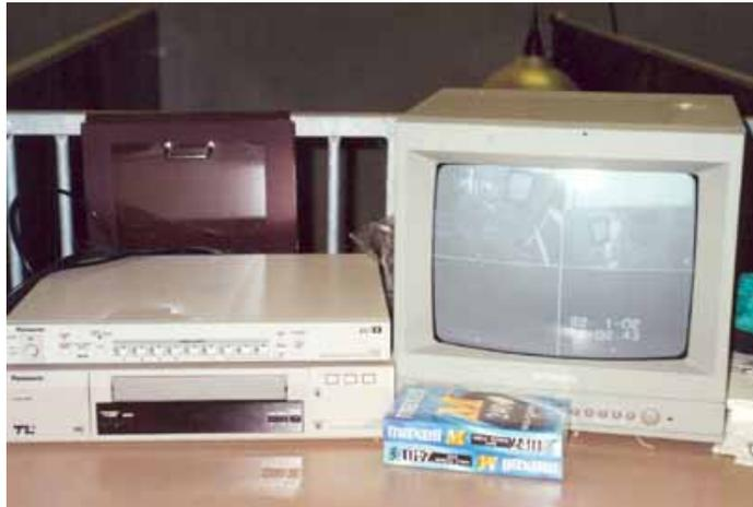
*Fig. 6.* Video cassette recorder and video multiplexer used for the recording of pig's behaviour.
