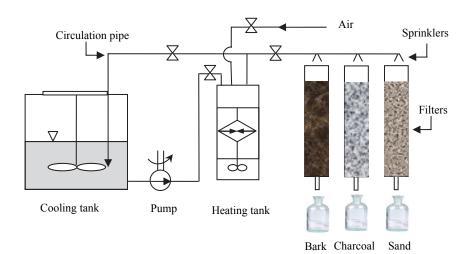
*Figure 1.* Schematic diagram of the greywater filter system used in all experiments (adapted from **Paper II**).
