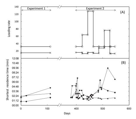
*Figure 6.* A) Hydraulic (L m<sup>-2</sup> day<sup>-1</sup>) ( $\circ$ ) and organic loading rates (g BOD<sub>5</sub> m<sup>-2</sup> day<sup>-1</sup>) ( $\times$ ) in the first (**Paper II**) and second (**Paper IV**) experiment. The truncation represents the periods when the filters were resting. B) Shortest residence time in the bark ( $\bullet$ ), charcoal ( $\blacktriangle$ ) and sand filters ( $\bullet$ ) during the different loading regimes.
