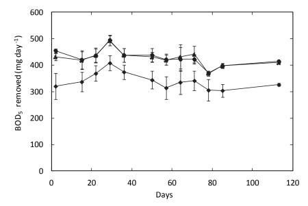
*Figure 2.* Amount of BOD<sub>5</sub> removed in the bark ( $\bullet$ ), charcoal ( $\blacktriangle$ ) and sand ( $\bullet$ ) filters loaded with artificial greywater at 15 g BOD<sub>5</sub> m<sup>-2</sup> day <sup>-1</sup> during 116 days (mean ± standard deviation; n = 2) (**Paper III**).
