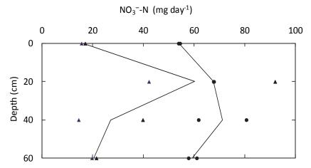
*Figure 4.* Profiles of NO<sub>3</sub><sup>-</sup>-N in infiltrated water in bark ( $\bullet$ ) and charcoal ( $\blacktriangle$ ) filters under greywater loading of 13-16 g BOD<sub>5</sub> m<sup>-2</sup> day<sup>-1</sup>. Lines represent mean values (n=2).
