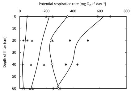
*Figure 3.* Potential respiration rate (mean, n =2) as a function of depth in bark ( $\bullet$ ), control bark ( $\circ$ ; n =1), charcoal ( $\blacktriangle$ ) and sand filters ( $\bullet$ ) at day 84 in the infiltration experiment with artificial greywater (**Paper III**).
