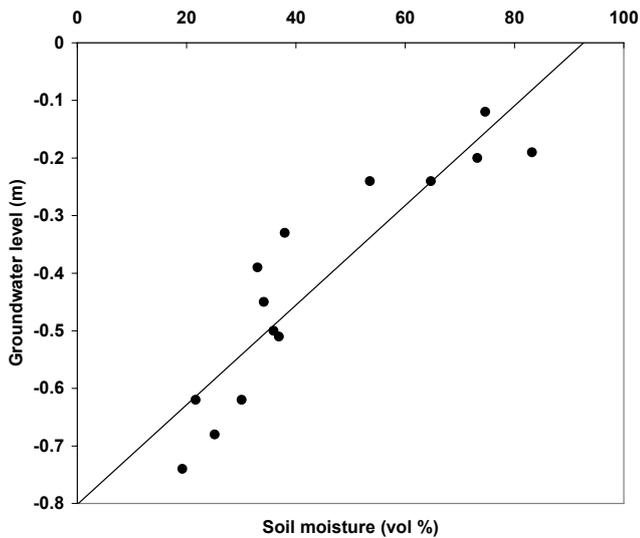
**Fig. 1.** Relationship between soil moisture (measured with TDR) and groundwater levels at the HP site in July 2002. Observations of both variables were available for 14 plots ( $r^2=0.823$ ,  $P>0.001$ ,  $n=14$ ).
