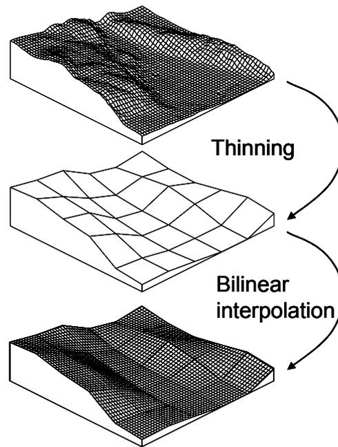
**Fig. 1.** Illustration of the extraction of lower resolution DEM from the original 5 m DEM by thinning, and the bilinear interpolation back to 5 m. Note the lower information content in the interpolated DEM.
