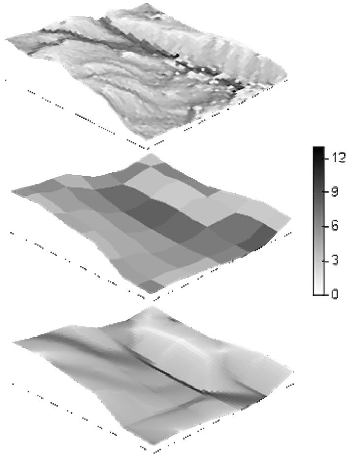
**Fig. 4.** Example from the maps of the specific upslope area,  $\ln(a)$ , for  $T_5$ ,  $R_5$  and  $T_{50}$ . (500 by 500 m window)
