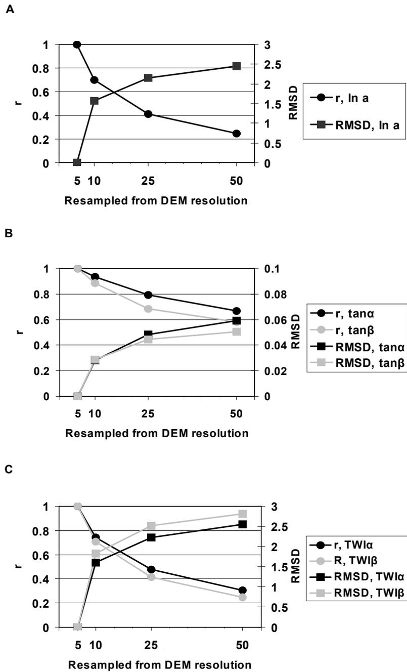
**Fig. 9.** Cell by cell correlation for a) specific upslope area, b)  $\tan\alpha$  slope and  $\tan\beta$  slope, c)  $TWI_\alpha$  and  $TWI_\beta$ .
