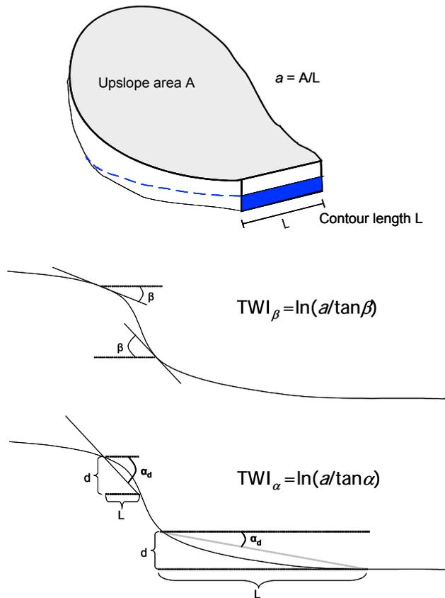
**Fig. 1.** The components of the TWI; specific upslope area  $a$ , local slope index ( $\tan\beta$ ) and downslope index ( $\tan\alpha=d/L$ ).
