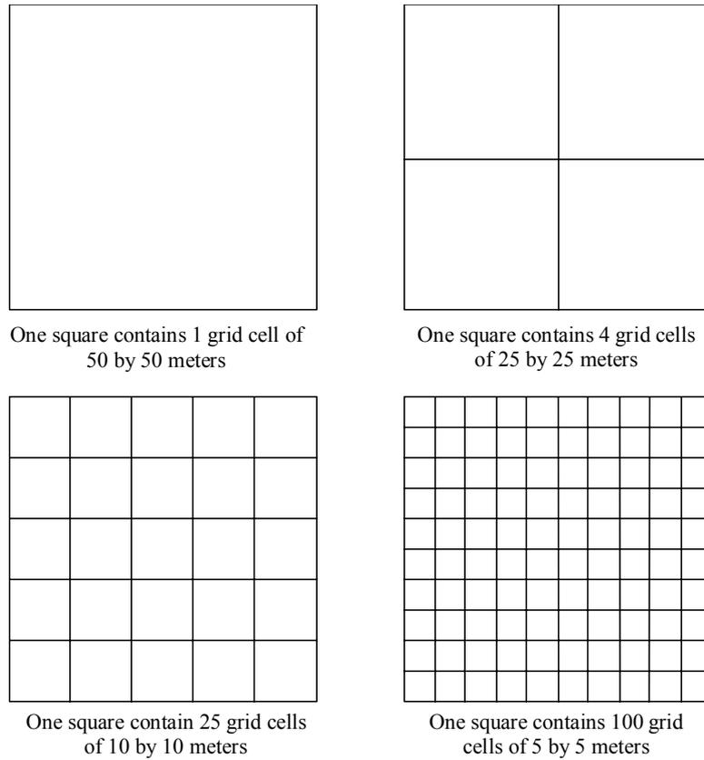
**Fig. 2.** The computed indices based on the DEMs  $T_{50}$ ,  $T_{25}$ ,  $T_{10}$  and  $T_5$  were compared based on squares of equal size. Each square contained a different number of grid cells in the different DEMs.
