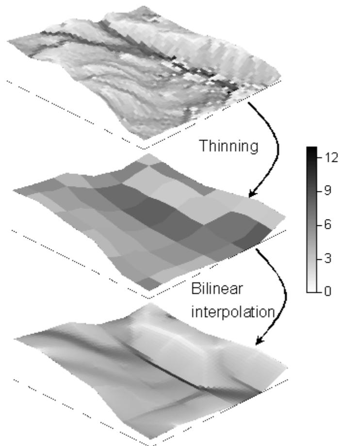
**Fig. 4.** Example from the maps of the specific upslope area,  $\ln(a)$ , for the original 5 m resolution DEM (above), a 50 m resolution DEM generated by thinning (middle), and a high resolution low information content DEM processed by bilinear interpolation back to 5 m resolution (below)(500 by 500 m window).
