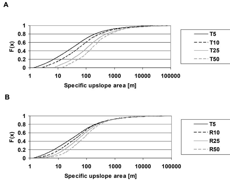
**Fig. 5.** Distribution functions for the specific upslope area a) for the lower resolution DEMs and b) for the resampled DEMs.
