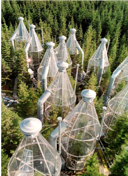
Figure 6. Picture and schematic diagram of the whole-tree chambers. (For a detailed description of the whole-tree chamber system showing the scale and describing all components outlined in the diagram, see Paper I, Fig. 1).
