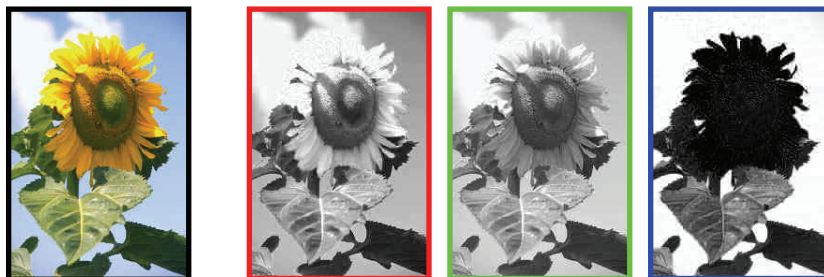
Figure 1 A typical digital color picture is a composite of three image channels representing red, green, and blue intensities.
