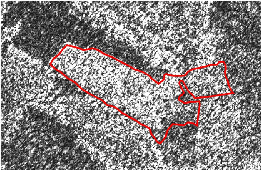
*Fig. 5.* A radar image from the airborne CARABAS-II VHF SAR sensor acquired at a flight altitude of about 3,400 m above ground, with a pixel size of 1 m. The imaged area covers about 600×400 m. Bright areas indicate high intensity (high stem volume) and dark areas low intensity (low stem volume) of backscattered energy.
