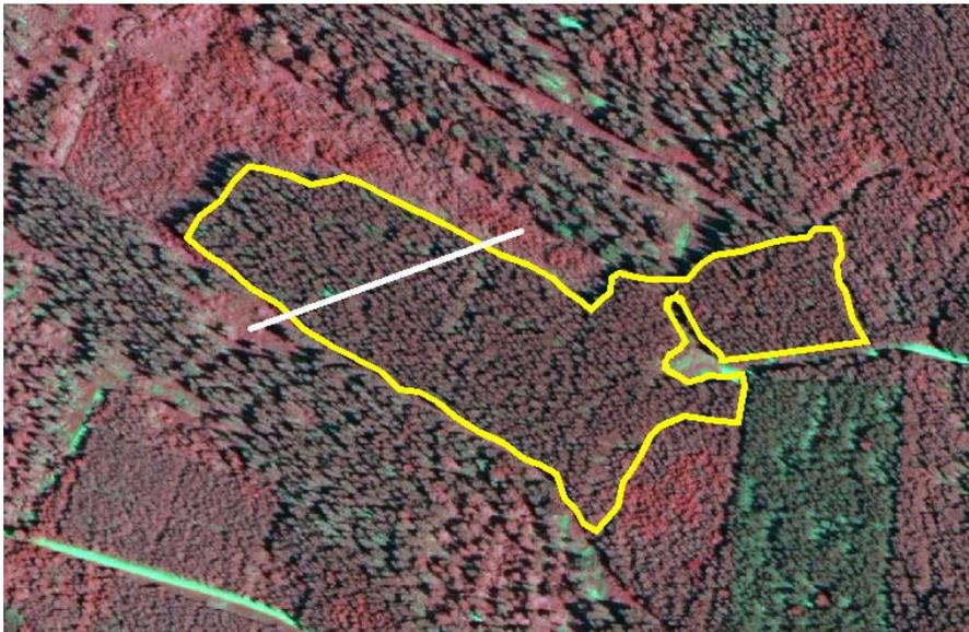
*Fig. 3.* A pansharpened color infrared image from the airborne Z/I DMC sensor acquired at a flight altitude of 4,800 m above ground, with a pixel size of 0.48 m. The imaged area covers about 600×400 m. The stand boundary, superimposed on the image, is outlined in yellow color. The white line shows the transect used to visualize laser data in Fig. 6.
