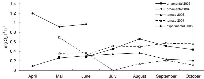
Figure 1: Oxygen consumption ( $\text{mg O}_2 \text{l}^{-1} \text{h}^{-1}$ ) of slow filters integrated to two commercial systems with tomato and ornamentals for 2004 and 2005. Displayed values for experimental systems are obtained 2005.
