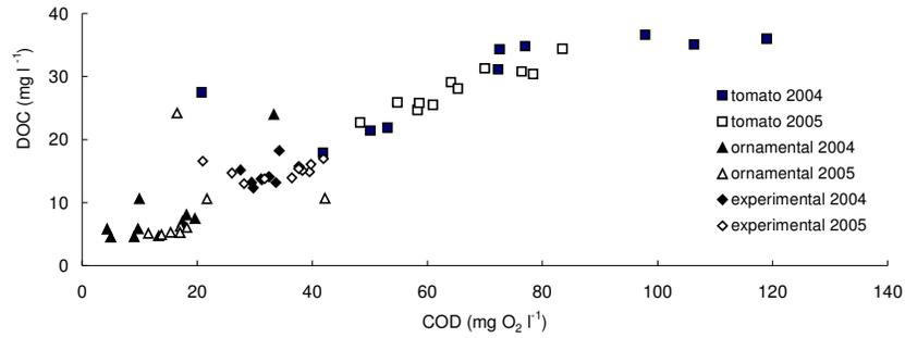
Figure 2: Mean values of DOC ( $\text{mg l}^{-1}$ ) and COD ( $\text{mg O}_2 \text{l}^{-1}$ ) in the supernatant of all systems in 2004 and 2005.
