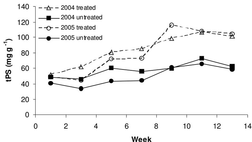
FIG. 1. Total polysaccharide content ( $\text{mg g}^{-1}$ ) in the filter skin of untreated and treated systems in 2004 and 2005. Measurements were made five days after inoculation of  $10.5 \text{ g}$  of FCWP  $\text{m}^{-2}$  to filters (treated) and continued for twelve weeks from early April until the end of June. Each data point represents the mean of three different systems, each connected to two slow filters ( $n=6$ ).
