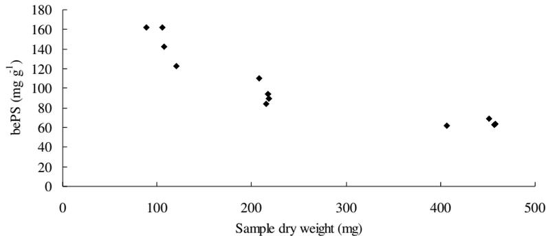
FIG. 2. Influence of sample dry weight on measured extracellular polysaccharide content (bePS) per g sample dry weight. Two samples with three different sample sizes each were collected from two different slow filters (n = 12).
