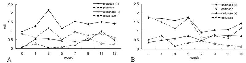
Figure 5: Dynamics in (A): protease and glucanase as well as in (B): chitinase and cellulase activities (mU) observed in filter skins of slow filters with (+) or without administration of fungal cell wall preparation (1.75 g FCWP per week) in 2005. Treatment started early April (week 1) and was conducted till end of June. Week 0 served as a control (n=6).
