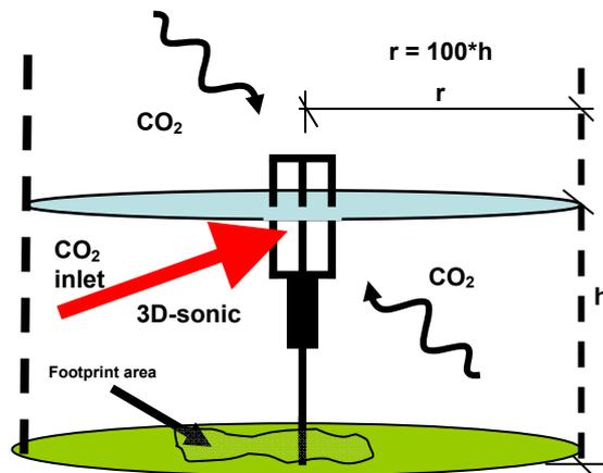
Figure 4 Schematic diagram of an Eddy Covariance system and its monitoring area.
