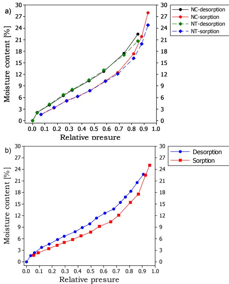
Figure 4 – Moisture sorption-desorption isotherms: a) *ncurri* and *ntholo*; b) Scots pine ( NC – *ncurri*; NT – *ntholo*)
