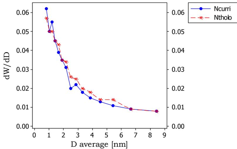
Figure 5 – Distribution of pore volume in pore sizes for ncurri and ntholo
