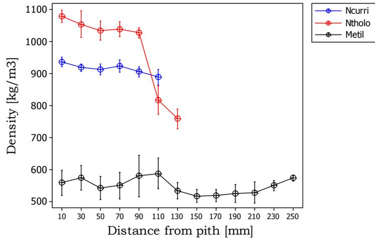
Figure 2 – Variation of density at 12% MC along radial direction at breast height of bole
