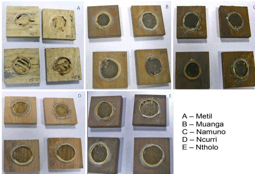
Figure 9 – Appearance of wood after termite test according to standard EN 118
