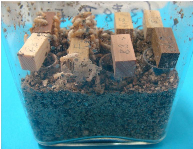
Figure 1 – Arrangement of wood specimens in a test vessel
