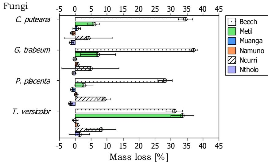
Figure 8 – Average and 95% confidence intervals of mass loss for the studied wood species after basidiomycete fungi test according to EN 113. Reference species: beech
