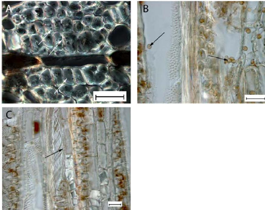
Figure 7 – Micrographs showing the decay features of ntholo sapwood after a soft rot test according to ENV 807. The arrows show typical cell wall cavities caused by soft rot (Fig. 7A), scattered spores that indicate fungal replication (Fig. 7B) and spirally oriented hexagonal cavities produced inside the cell wall (Fig. 7C). The bars correspond to 10  $\mu\text{m}$
