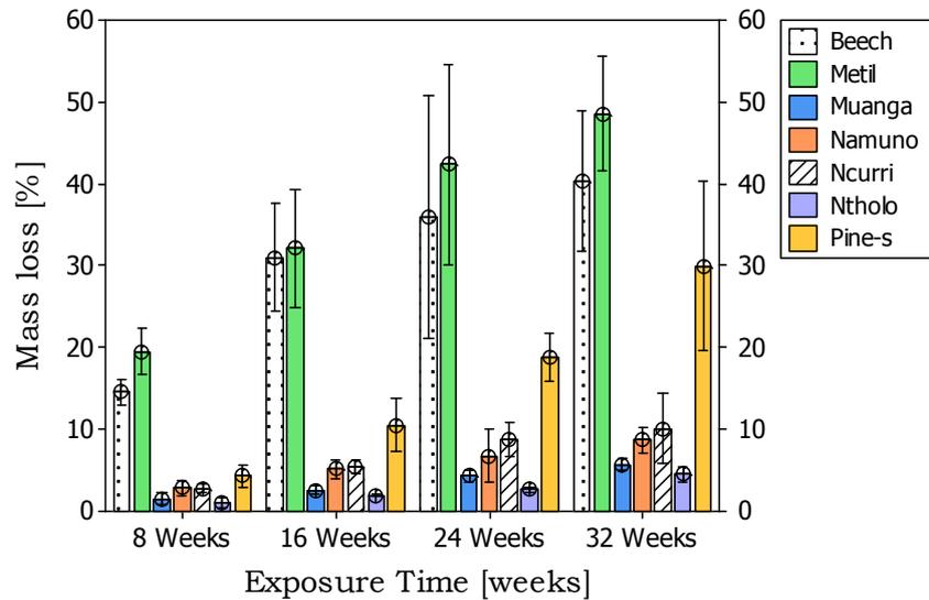
Figure 6 – Average and 95% confidence intervals of mass loss for the studied wood species after soft rot test according to ENV 807. Reference species: beech and pine sapwood
