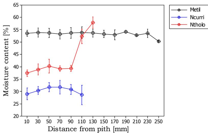
Figure 3 – Variation of green MC along the radial direction at breast height of a bole
