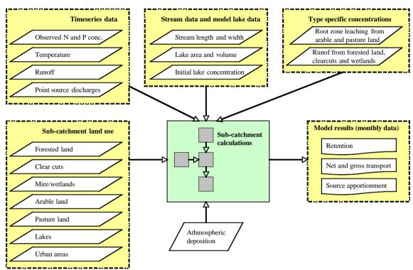
Figure 1. The general structure of inputs and outputs to the FyrisNP model.
