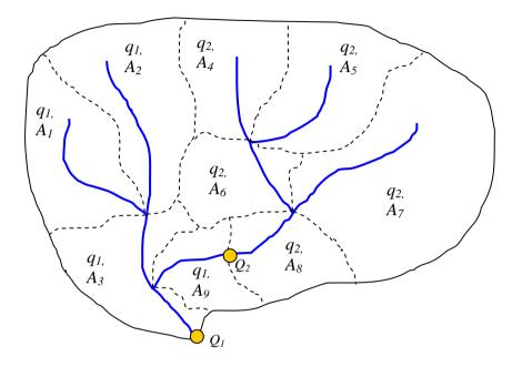
*Figure 2.* The areas (A), discharge measurement stations (Q), and area specific runoffs (q) within an example catchment.
