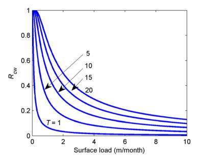
Figure 5. The retention coefficient,  $R_{cw}$ , as a function of surface load for various water temperatures. For all temperatures and surface loads,  $k = 0.069 \text{ m month}^{-1} \circ C^{-1}$ .
