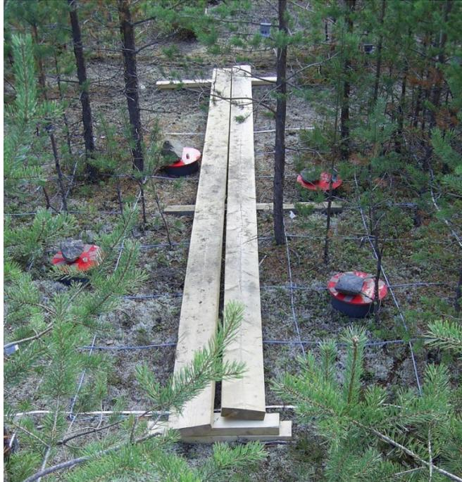
Figure 3. Opaque collars for sequential gas sampling of soil-respired CO<sub>2</sub> after labelling the canopy with <sup>13</sup>CO<sub>2</sub>.
