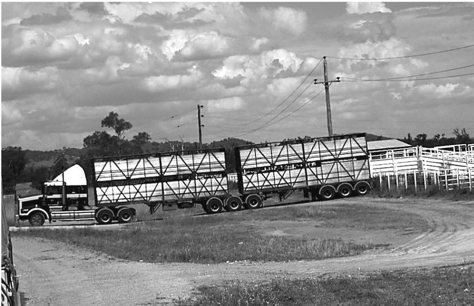
**Photo 3:** Australian enclosed transport vehicle with ventilation openings in the wall.
