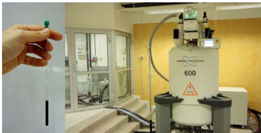
Figure 3. Glass tube containing an extract of a boreal forest humus soil (left) which is then inserted into the Nuclear Magnetic Resonance spectrometer (right) to obtain ^{31}\text{P} NMR spectra of soils. Photo Andrea Vincent.
