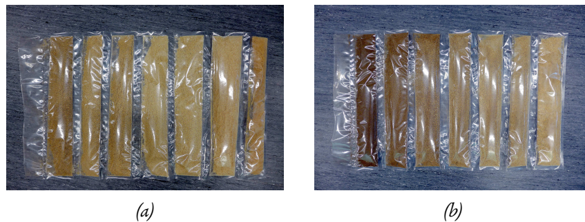
Figure 9: Milled and sealed samples for analysis of ash content (a) Energy wood (b) Stored logging residues.
