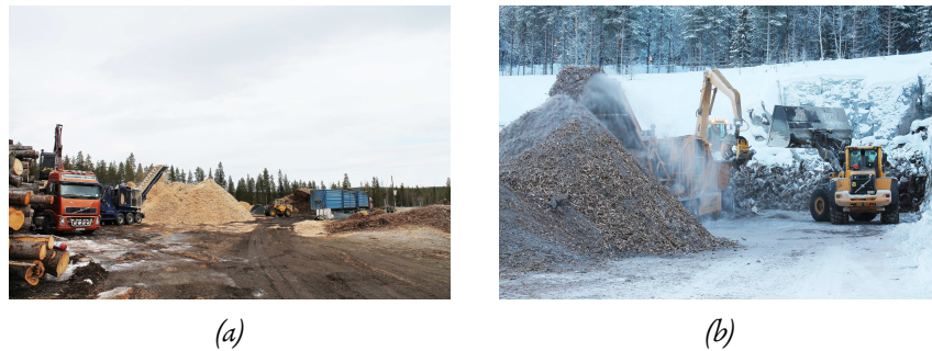
Figure 5: (a) Energy wood loaded by truck mounted crane into Petersson chipper (b) Stumps loaded by grapple and front end loader into CBI Magnum Force crusher.
