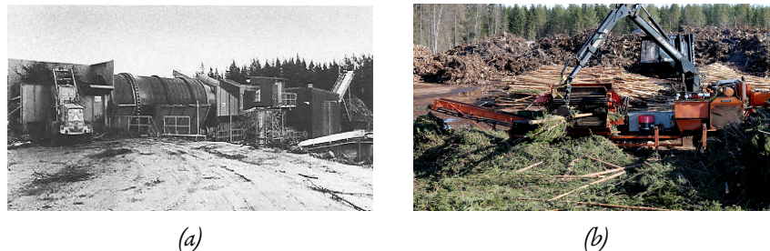
Figure 4: (a) A delimiting drum at the forest biomass terminal (Photo: Jonas Palm) (b) Chain flail delimiting at the terminal operations.
