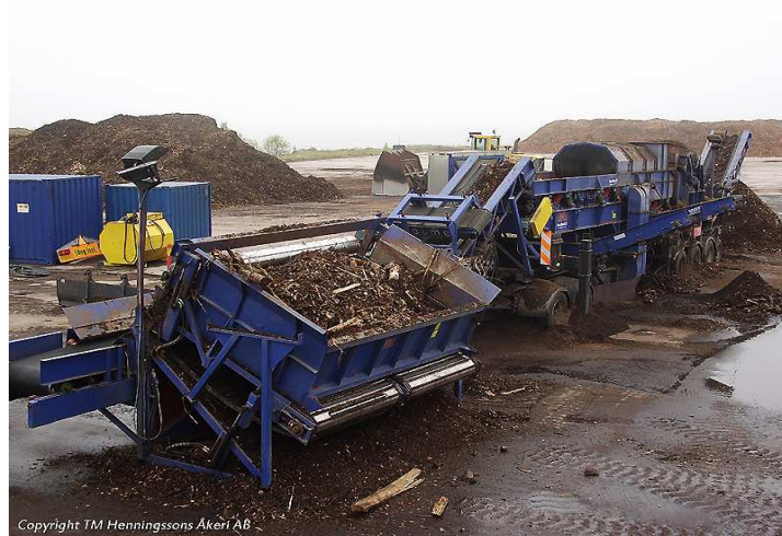
Figure 16: Bark screening with a mobile machine at a terminal in northern Sweden ©TM Henningssons Åkeri AB.
