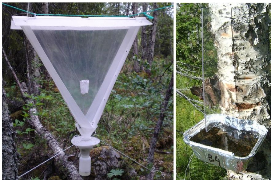
Figure 2. To the left: IBL2-trap. To the right: trunk-window trap.
