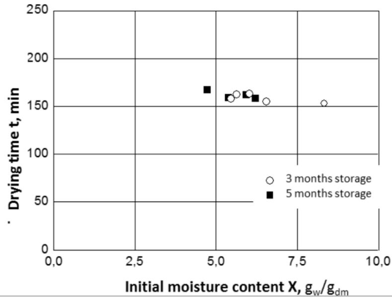
Figure 1.1.5 Drying time of apple slices down to a final moisture content of 0.13 gw/gdm related to initial moisture content. Drying conditions like in Figure 3
