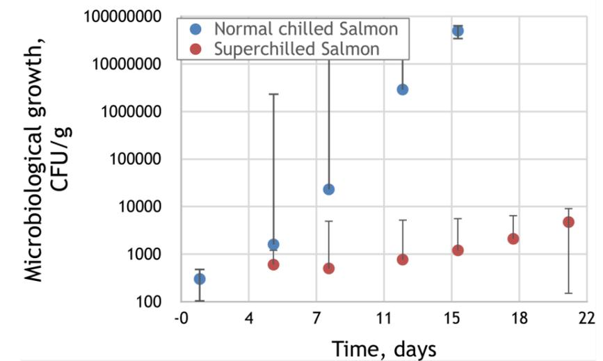
Figure 2.2.2: Number of colony forming units (CFU) in salmon filets during storage of fresh, chilled and superchilled salmon filets processed after Method 1, with ice level of 15% (red) stored at -1.5°C, and chilled reference samples stored at +3°C (blue)
