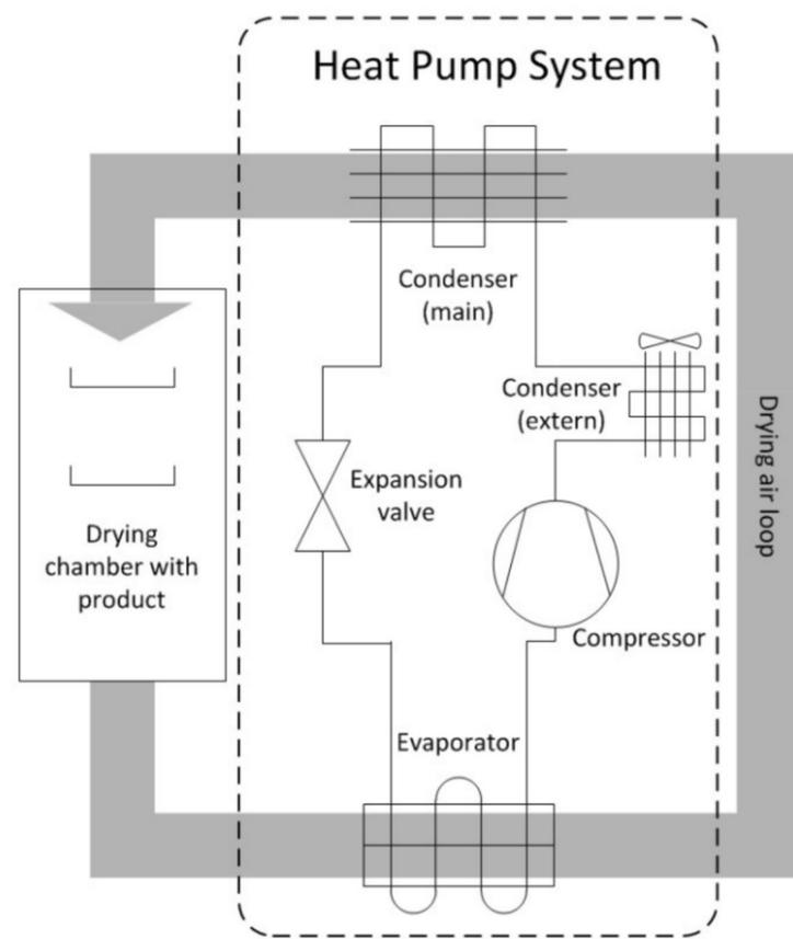
Figure 5.3: Principal layout for heat pump assisted drying for convective (air) drying in closed loop.
