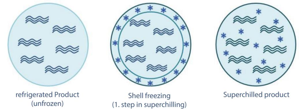
Figure 1.4: The different steps in superchilling of food: The present water in the product is partially frozen and after a certain time mixture of water and ice is present inside the structure of the product.
