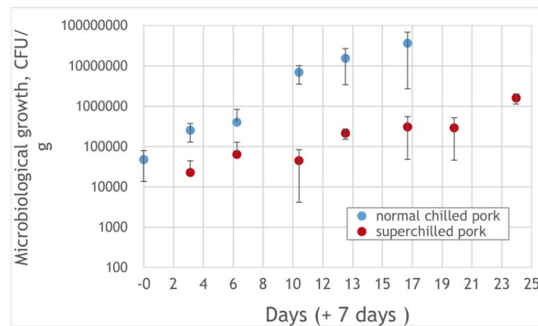
Figure 2.2.7: Number of colony forming units in pork with ice level of x (red) and chilled reference sample at +3°C during storage
