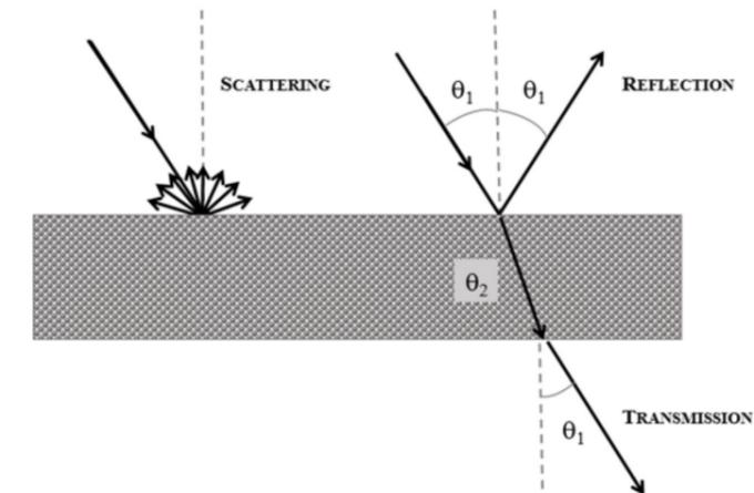
Figure 6.2: Interaction between matter and electromagnetic radiation (Raponi et al., 2017)
