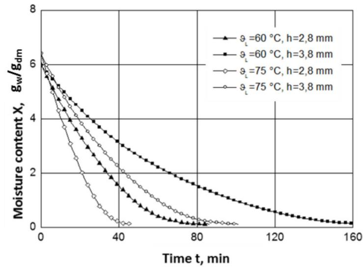
Figure 1.1.2: Drying behaviour of apple slices of different thicknesses at different drying parameters: 60 °C air temperature (air velocity 3.4m/s, dew point 17.5 °C), 70 °C air temperature (air velocity 4.3 m/s, dew point 17.5 °C)
