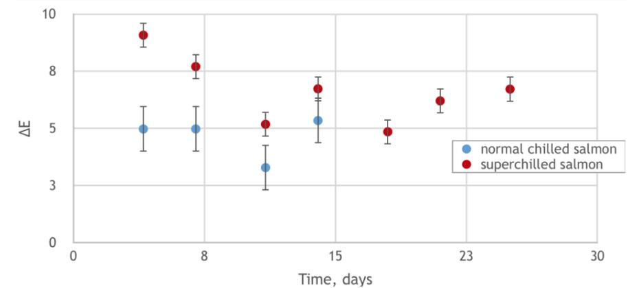
Figure 2.2.5: Colour changes  $L^*a^*b$  (expressed as delta E) for normal chilled and super-chilled salmon fillets with ice level of 15% (red) stored at -1.5°C, and chilled reference samples stored at +3°C (blue).
