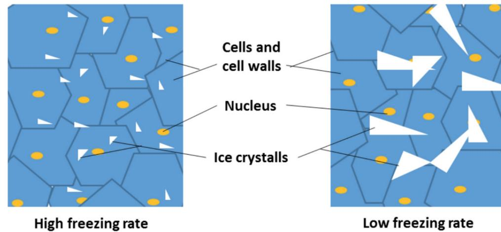
Figure 4.2: Crystal growth depending on freezing speed
