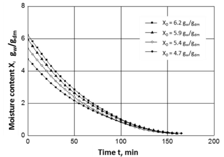
Figure 1.1.4: Drying behaviour of apple slices with different initial moisture content (after 5 months storage) dried at 60 °C (air velocity = 3.4 m/s, dew point = 17.5 °C)
