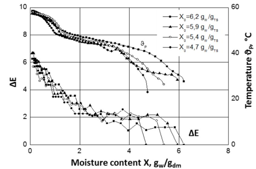
Figure 1.1.7: Product temperature and colour change  $\Delta E$  for different initial moisture contents  $X$  as a function of moisture content, drying conditions like in Figure 3
