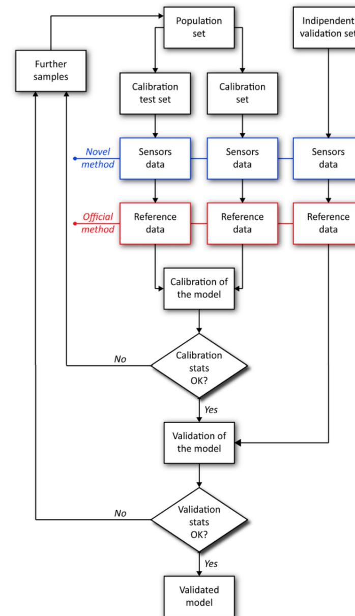
Figure 6.6: Workflow of data pre-processing, calibration and validation steps
