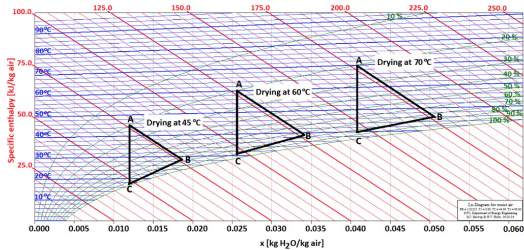
Figure 5.4: Mollier-diagram for the drying process at the different temperatures, where A denotes the inlet to the drying chamber, B the outlet and C the state after vapour condensation before reheating. For drying at 70 °C these states were at point A: 20 % relative humidity and 70 °C; point B: 75 % relative humidity and 46.4 °C and point C: nearly saturated at 39.4 °C.
