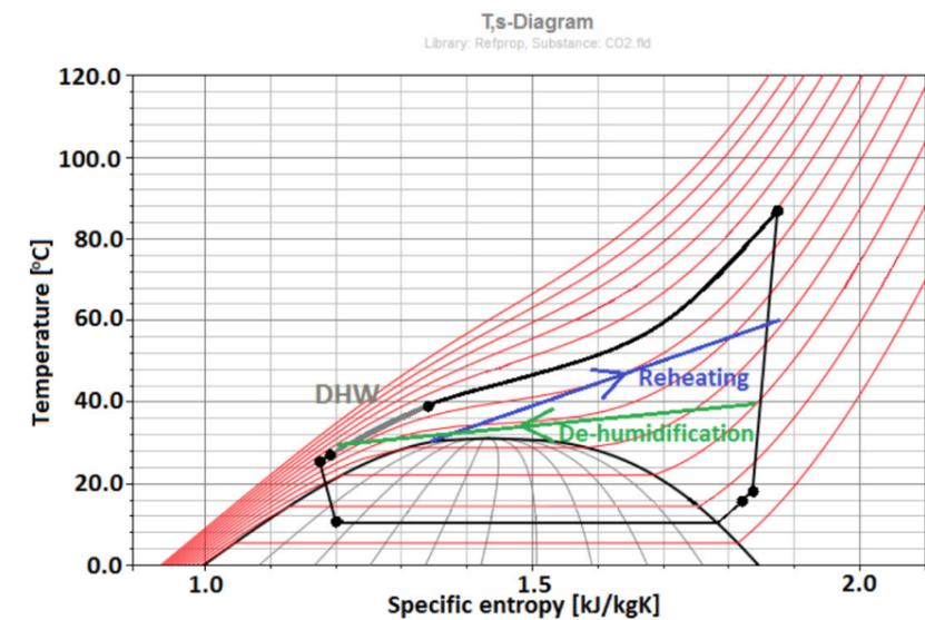
Figure 5.6: Heat pump assisted drier with R744 for drying temperature of 60°C.
