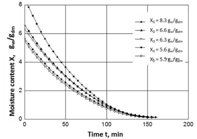
Figure 1.4 shows the drying curves for apples dried stored for 5 months. Like for the previous mentioned apples, the required moisture content was almost achieved at the same time. Further, it is shown that apples stored for a longer time have lower initial moisture contents, which means they significantly lose water during storage.
