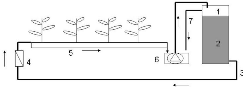
Figure 1. Schematic view of the system used for greenhouse experiments. 1) Water supernatant 2) Filter column 3) Outflow from filter 4) Flow meter 5) NFT-gutters with plants 6) Reservoir with plunger pump 7) Overflow.
