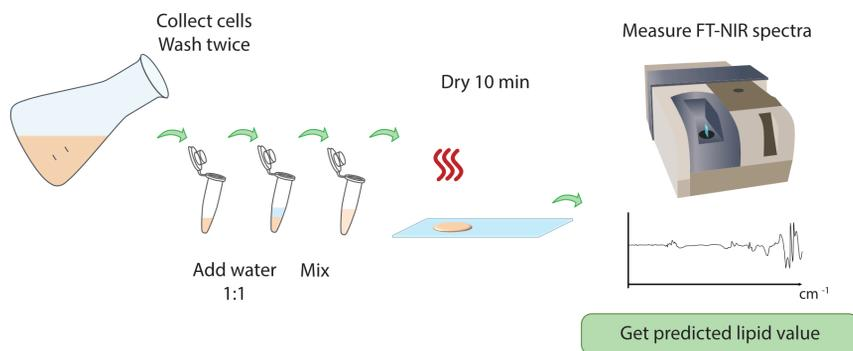
Figure 13. Sample preparation for Fourier transform-near infrared (FTNIR) lipid prediction.
