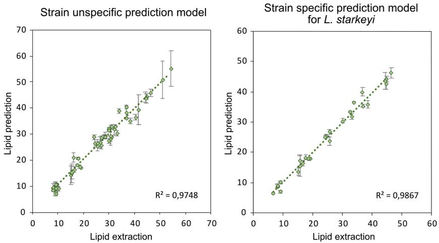
Figure 14. Calibration of two Fourier transform near infrared (FTNIR) lipid prediction models. (Left) A strain-unspecific lipid prediction model and (right) a lipid prediction model for *Lipomyces starkeyi*.
