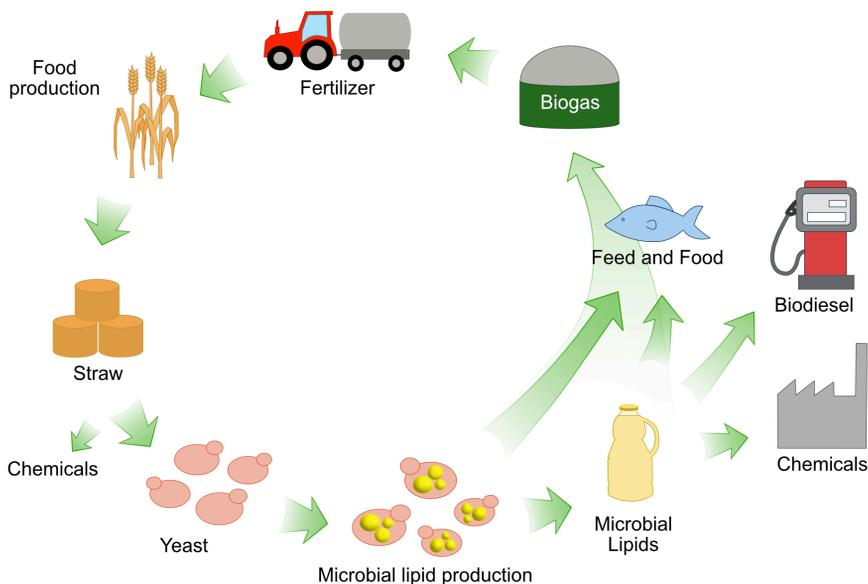
*Figure 1.* Sustainable microbial lipid production for fuels, chemicals or food and feed production in a circular biorefinery approach where wheat straw is used as a substrate for microbial lipid production with yeast. Recycling the residues for biogas and the biodigestate as fertiliser closes the circle.
