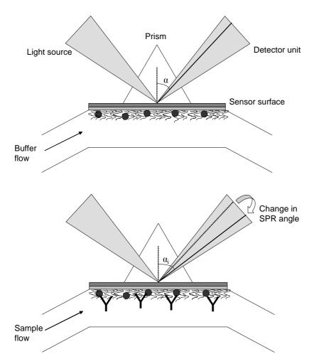
*Figure 2.* The optical detection system used in the Biacore instrument. Upon binding or dissociation of molecules to the sensor surface the refractive index near the surface changes, resulting in a shift in the SPR angle ( $\alpha$ ).
