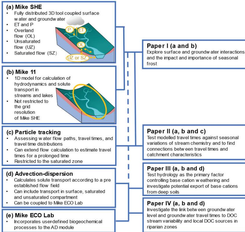
Figure 2. A schematic figure of model tools and applications. The figure shows the model tools used, the main usages for each tool and which were used in each paper of this thesis. The tools shown are (a) Mike SHE, (b) Mike 11, (c) Particle tracking (d) Advection-dispersion and (e) Mike ECO Lab.
