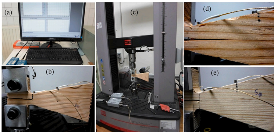
Fig. 9. The experimental setup for fracture monitoring under mechanical loading using the AE technique. The setup was designed for the mode I fracture test to study the crack tip propagation in the double cantilever beam (DCB) specimen while the sample geometry provided stability of energy release rate during the crack growth process (a) AE equipment (b) DCB specimen (Douglas fir) (c) mechanical testing machine (d) crack tip propagation (e) DCB specimen (white fir) [45].
