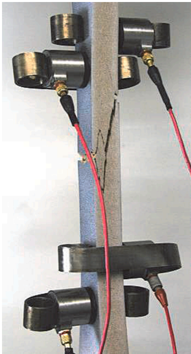
Fig. 10. AE sensors for detecting crack location during mechanical (tensile) loading of wood-based composite. The experimental setup with four AE sensors was designed to allow for a simplified linear location between AE sensors placed on each panel plane [105].
