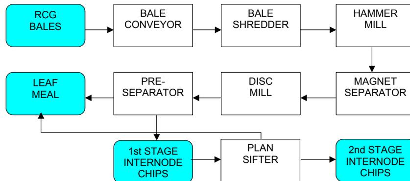
Figure 3. Schematic overview of the dry fractionation process developed by UMS A/S.
