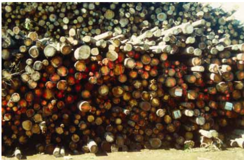
Fig. 7. The experimental logs (the upper layer marked with red) in the experimental pile after 8 weeks of sprinkled storage.
