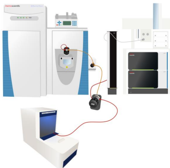
Figure 3. An example of a set up for running EDA based on HPLC (top left), HRMS (top right), and fractionation into 96-well plates using a FractioMate™ (bottom). The well plates are then used for bioanalytical analysis.
