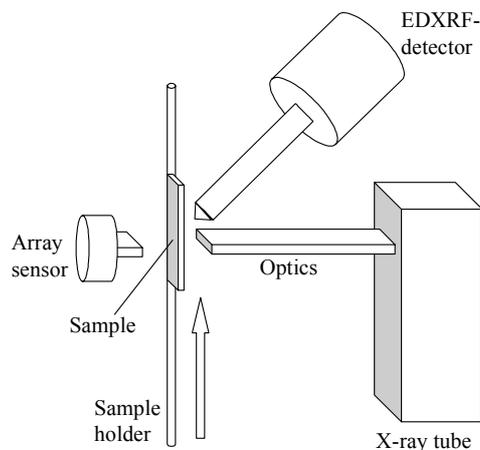
Fig. 3. Devices set-up in the Woodtrax.
