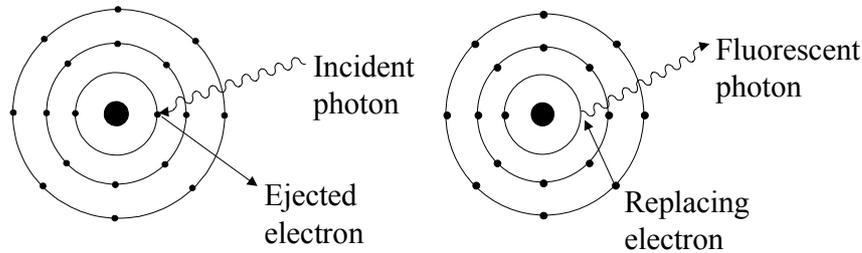
*Fig. 1.* Photoelectric absorption of a photon followed by the formation of a fluorescent photon.
