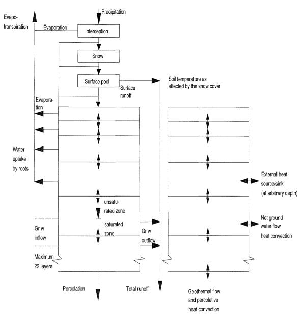
Mass balance (left) and heat balance (right) of the SOIL model.
