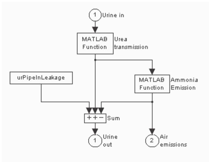
Figure 17. The urine-pipe sub-model.
