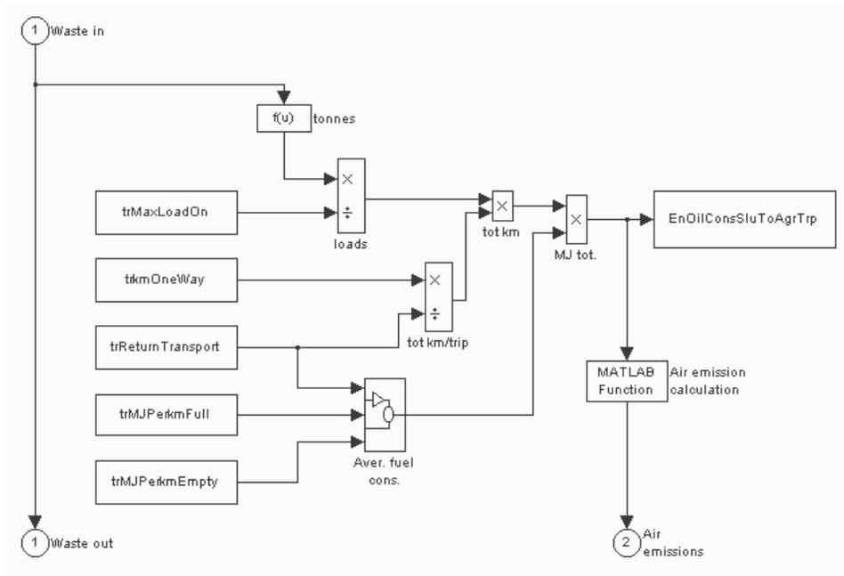
Figure 19. The truck sub-model.
