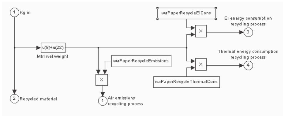
Figure 62. Paper recycling sub-model.
