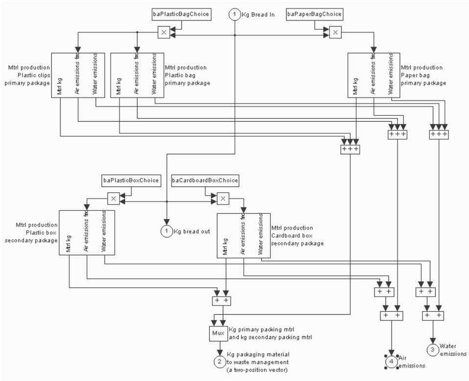
Figure 59. The sub-model for choices of primary and secondary packaging.
