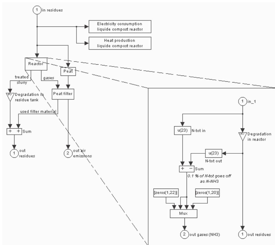
Figure 16. The liquid compost sub-model.
