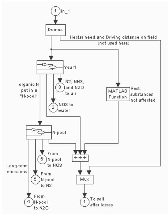
Figure 22. The soil nitrogen turnover sub-model.
